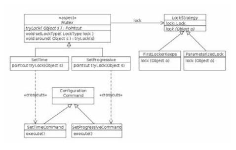
Figure 6.8: Class diagram for mutex interaction implemented in Aspect J.
