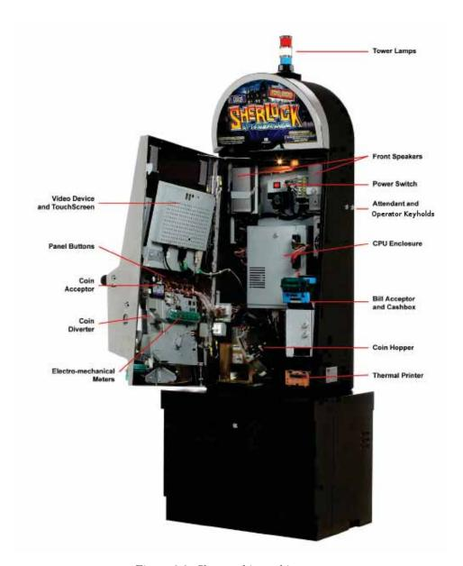
Figure 3.3: Slot machine cabinet
