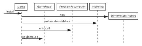
Figure 6.3: Sequence diagram for Demo aspect installation in PHANtom.
